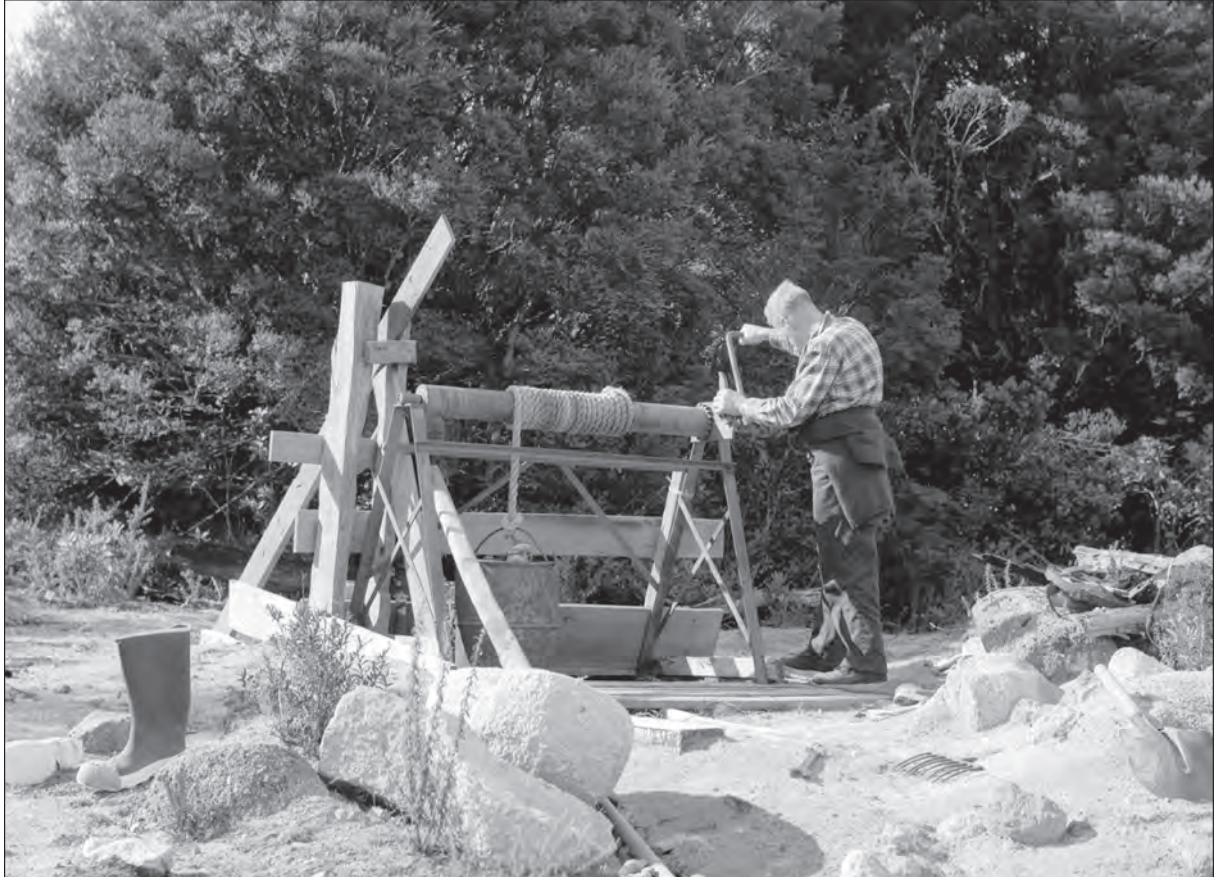
A windlass is cheap and easy to build and can be used to raise or lower men, equipment, water and stone. Image courtesy of TAHO and not from the Sentinel claim.
